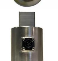
Euroload Limited provide a range of torque load cells. The 7000 NM torque load cell is a stock item. The 2"(50.8mm) male analyser is manufactured from high grade stainless steel with mil-spec connections for use in ROV buckets.
