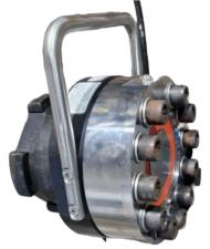
Euroload Limited low profile pancake load cells have been designed for the harshest of environment's for multiple applications including, silo content's monitoring, hydraulic ram verification, test frames and many more. Our clients fit this cell into Linear Valve Override tool verification buckets to accurately verify the load produced from their subsea intervention tools.
