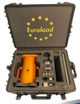
Euroload Limited provide a range of telemetry torque Verification tools kits.
